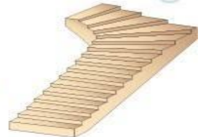
Combined ladder (L-span, bending from the top)
